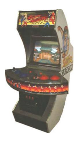
Instead of traditional buttons, Street Fighter featured two large 'punch pads' for its punch and kick buttons. While they were pressure sensitive (a lighter hit produces a Jab punch or a Short kick, whereas harder hits produce heavier attacks) they were also notorious for breaking too easily. Which eventually prompted Capcom to abandon the 'Punch Pads' idea in favor of the more infamous six button layout.
